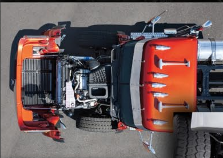
Hood tilts to approximately 90 degrees for easy engine and fluid access.
