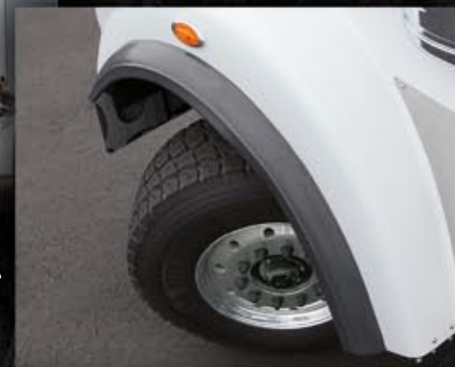
Wheel cut up to 50 degrees for excellent maneuverability.
