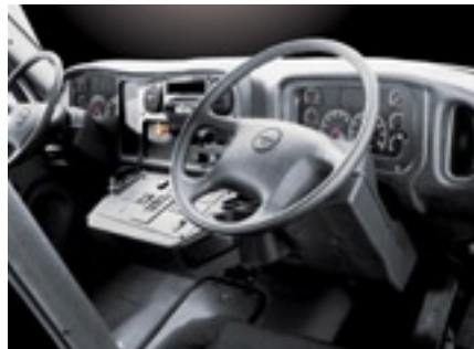
Interior of the Business Class M2 106 featuring the Sit-Down Dual Drive Option.
