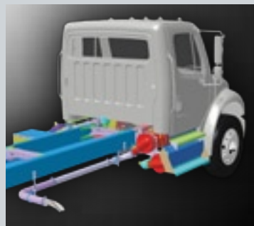
CURBSIDE EXIT TAILPIPE
